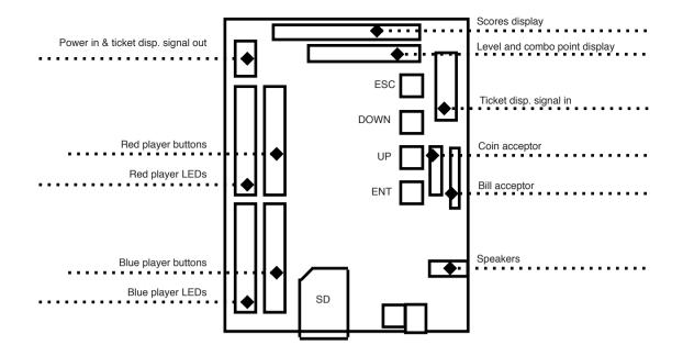
**Notice:** if machine runs out of tickets while dispensing them, open the machine, insert more tickets and press ESC on the main board to resume dispensing tickets.
